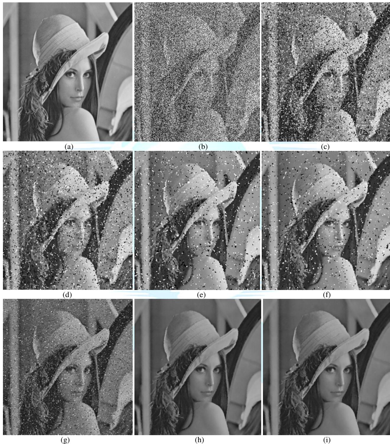
Figure3: Restoration results of different filters (a) Original test image "Lena" (b) Corrupted image with 60% salt & pepper noise(c) Median filter with 3 X 3 window size (d) CWM filter with 3 X 3 window size & center weight of 3(e) Iterative Median filter with 3 X 3 window size & 3 iterations (f) Iterative Switch Median filter (g) Improved Progressive Switching Median filter. (h) Simple Adaptive Median Filter (i) Proposed Filter
